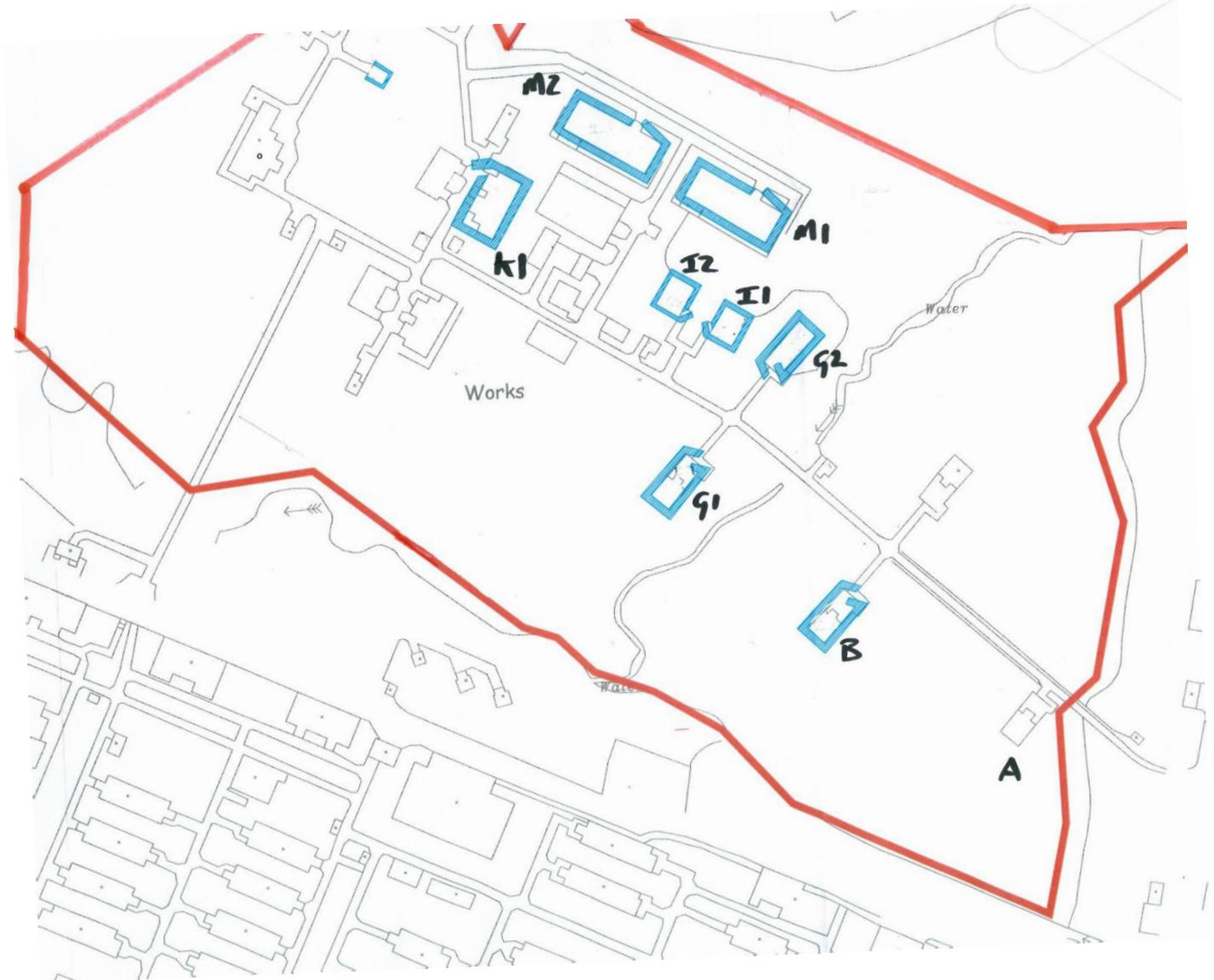
Note on this example, the red line indicates the extent of the licensed site, the blue line indicates buildings licensed for the presence of explosives and the letters refer to building details that would be contained within a separate schedule.
